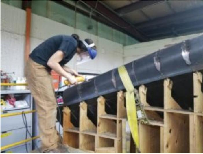
*Jane Thompson grinding the weld so it is flush to the surface. The project required all visible welds to be ground.*
